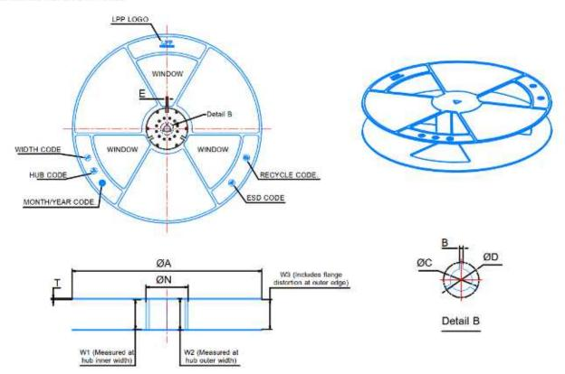
MATELIAL: ANTISTATIC POLYSTYRENE (Surface resistance10E5</= X </=10E10)
